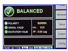
The instrument also measures the true test circuit burden as seen by the transformer-under-test. Knowing the true burden can facilitate a resolution to commonly encountered measurement anomalies and also ensure that the transformer is being tested at the appropriate burden operating point. The burden is displayed as VA (volt-amperes) and PF (power factor).
